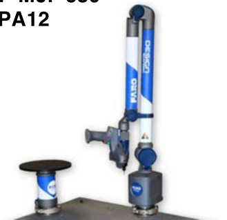
FARO Design Scan Arm (Scanner 3D + Palpeur)
